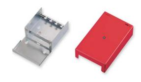
Description Delivery **Order Number** Metal Outlet, 4-Port, 45 x 93 x 143.5 mm (HxWxD), for the installation of 4 LANscape modules, straight, metal construction with integrated strain relief, patchcord protection and excess length storage for FO cables anthracite, RAL 7016 1/1 WAXWSD-U0408-C001
