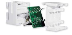
Disassembled S250 Basic Module
